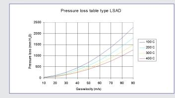
advise in detail and make computer calculations. Temperature Maximum: 600°C. Special designs are available for higher temperatures.
